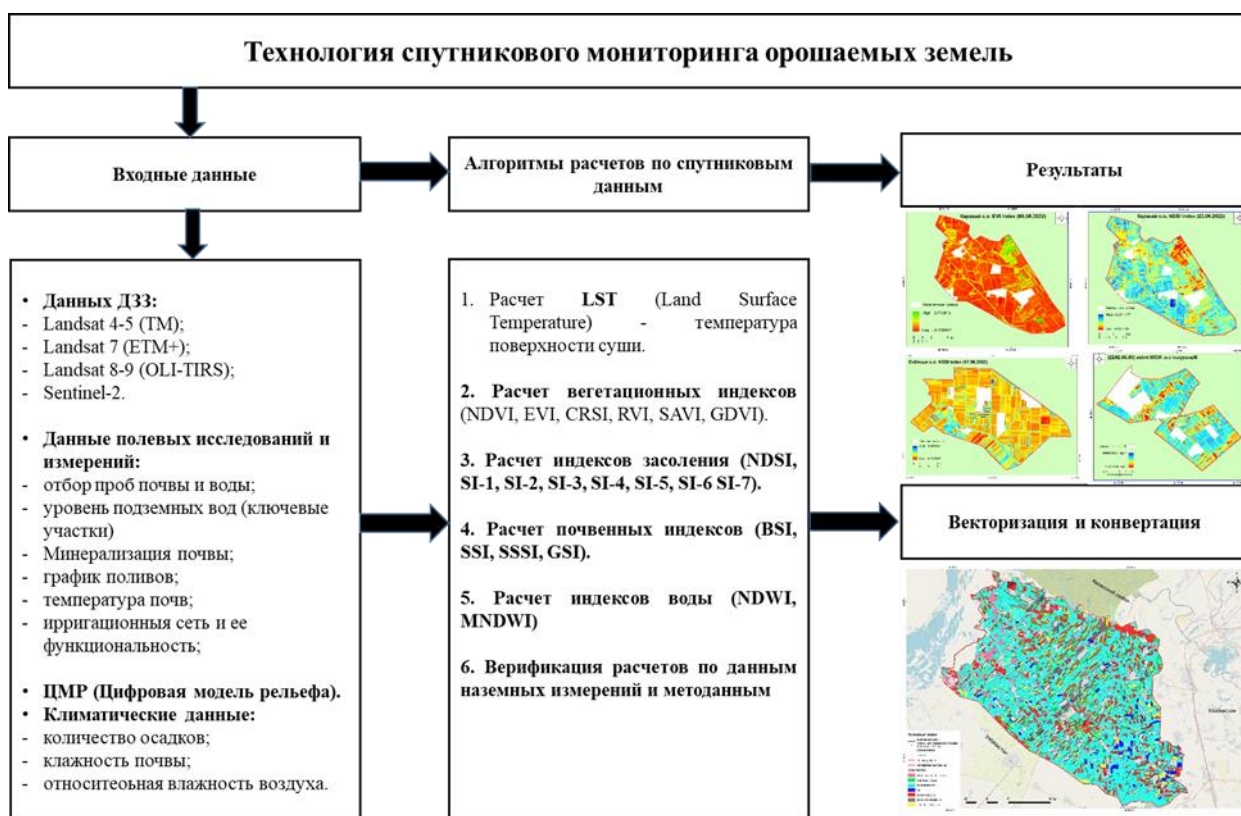
Figure 1. Methodology for assessing and mapping degradation processes in irrigated lands based on remote sensing technology
